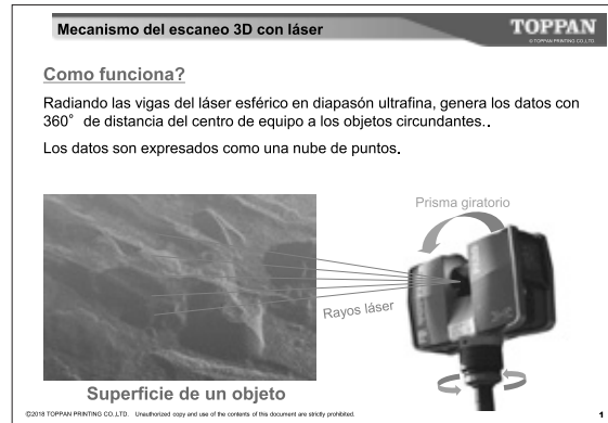
Fig. 10. 3D laser scanning equipment: FARO Focus 3D X330HDR (Courtesy of Toppan Printing, Co. Ltd.).
