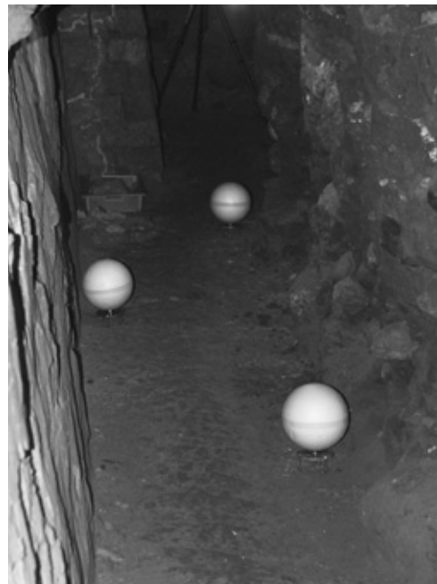
Photograph 10. Markers (targets) situated inside one of the PIAT tunnels.
