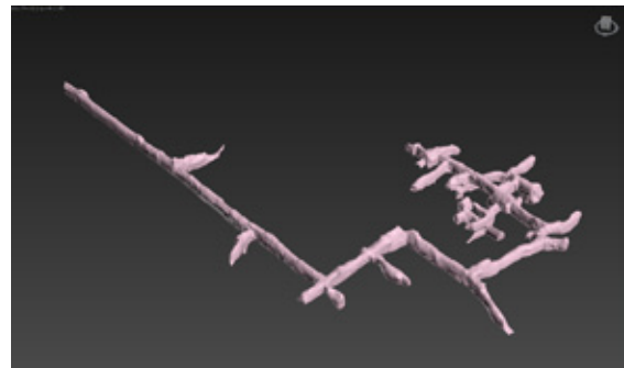
Fig. 14. Tunnel network after polygonalization.
