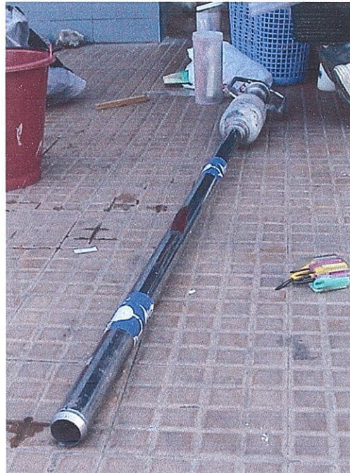
Photo 20: A Phleger type gravity core sampler.
