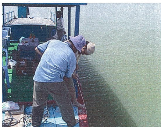
Photo 7. Onboard settlement of a Phleger type core sampler on the Tonle Sap River, off Kompong Chhnang
