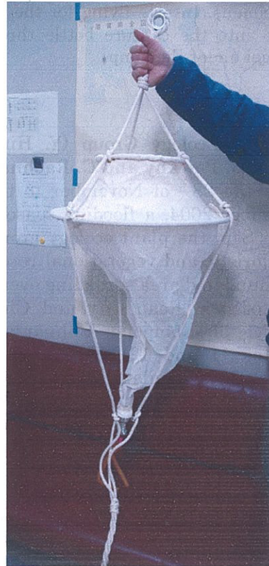
Photo 9: Double netting plankton net. A special plankton net with double fine-mesh netting cloth. Inner net with 100 \mu m aperture collects larger plankton, mostly zooplankton. Outer net with 50 \mu m aperture collects smaller plankton, mostly phytoplankton.
