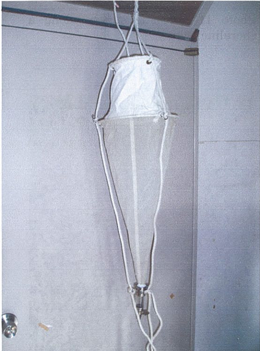
Photo 8: Plankton net, for collecting zooplankton staying water column quantitatively. The fine mesh (70 \mu m) filtrate water when the net is hauled with the linked rope.
