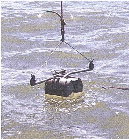
Photo 19: A grab sampler type DIK-140.
