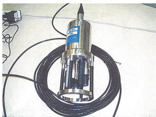
Photo 13: The multi-parameter water quality profiler.
