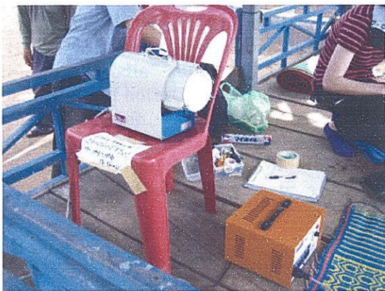
Photo 9. Air sampling using a portable high-volume air sampler near the western approach of Angkor Vat, Siem Reap
