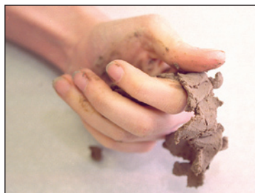
Figure A5. Class III soil (Silty clay loam—31 percent clay, 18 percent sand, 51 percent silt).
