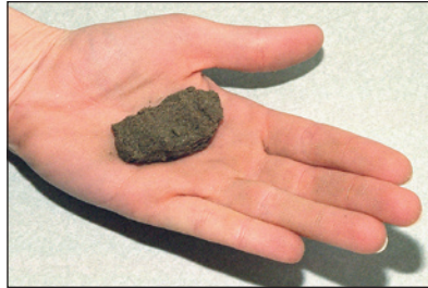
Figure A1. Class Ib soil (Loamy sand—2 percent clay, 85 percent sand, 13 percent silt) forming a cast.
