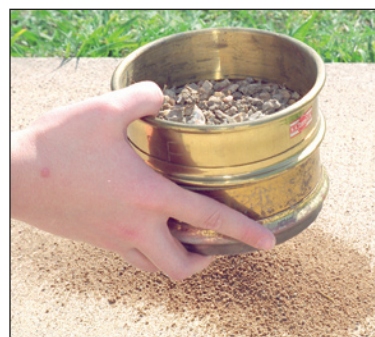
Figure 6. Particle size separation using a number 4 sieve on top of a number 10 sieve.
