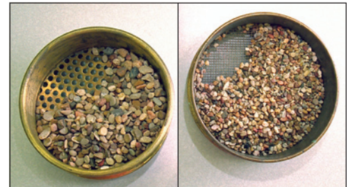
Figure 3. Number 4 sieve (left) with particles larger than 5 mm and number 10 sieve (right) with particles larger than 2 mm but smaller than 5 mm.
