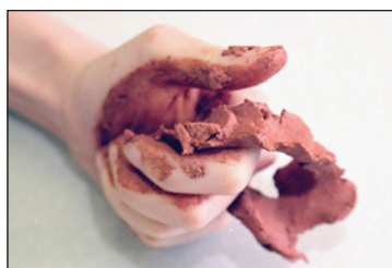
Figure A7. Red Class IV soil (Silty clay—48 percent clay, 6 percent sand, 46 percent silt).
