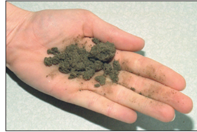
Figure A2. Dropped cast of Class Ib soil (Loamy sand—2 percent clay, 85 percent sand, 13 percent silt).
