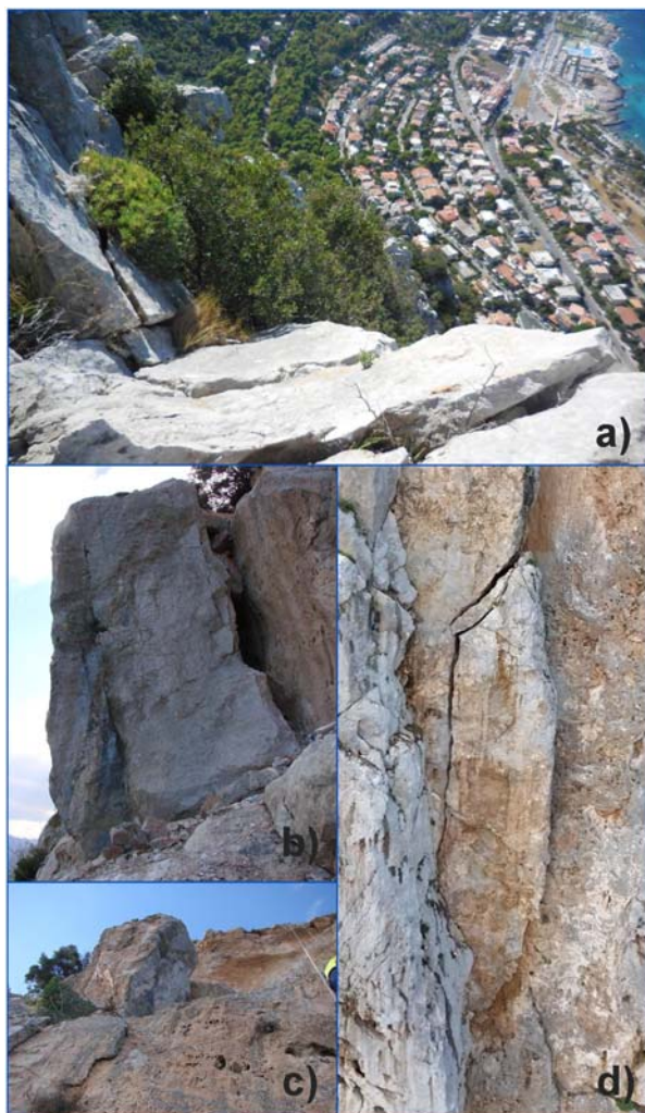
Figure 5. Unstable blocks as a. slabs, b.,c.boulders and d. pinnacles which could involve in kinematics of toppling.
