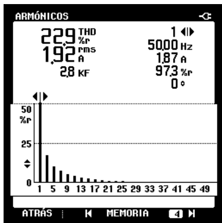
Fig. 10. Measurements of the load voltage v_L and current i_L before compensation, for the Current Rectifier load case: a) waveforms, b) active, reactive and apparent powers, c) voltage harmonic spectrum, d) current harmonic spectrum.
