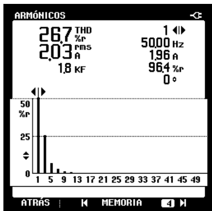
Fig. 7. Measurements of the load voltage v_L and current i_L before compensation, for the Voltage Rectifier load case: a) waveforms, b) active, reactive and apparent powers, c) voltage harmonic spectrum, d) current harmonic spectrum.
