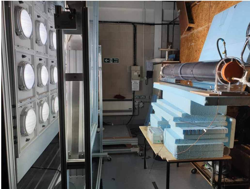
Figure 7. Indoor solar thermal simulator experimental setup and testing.
