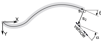
Figure 4. Vehicle positioning through curvilinear coordinates, adapted from [16].
