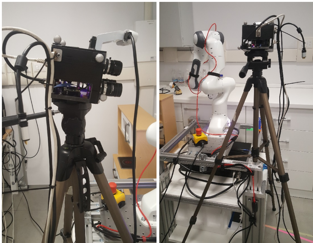
Figure 4.2: The custom setup endowed, among other sensors, with event-based cameras and the Panda robot.
