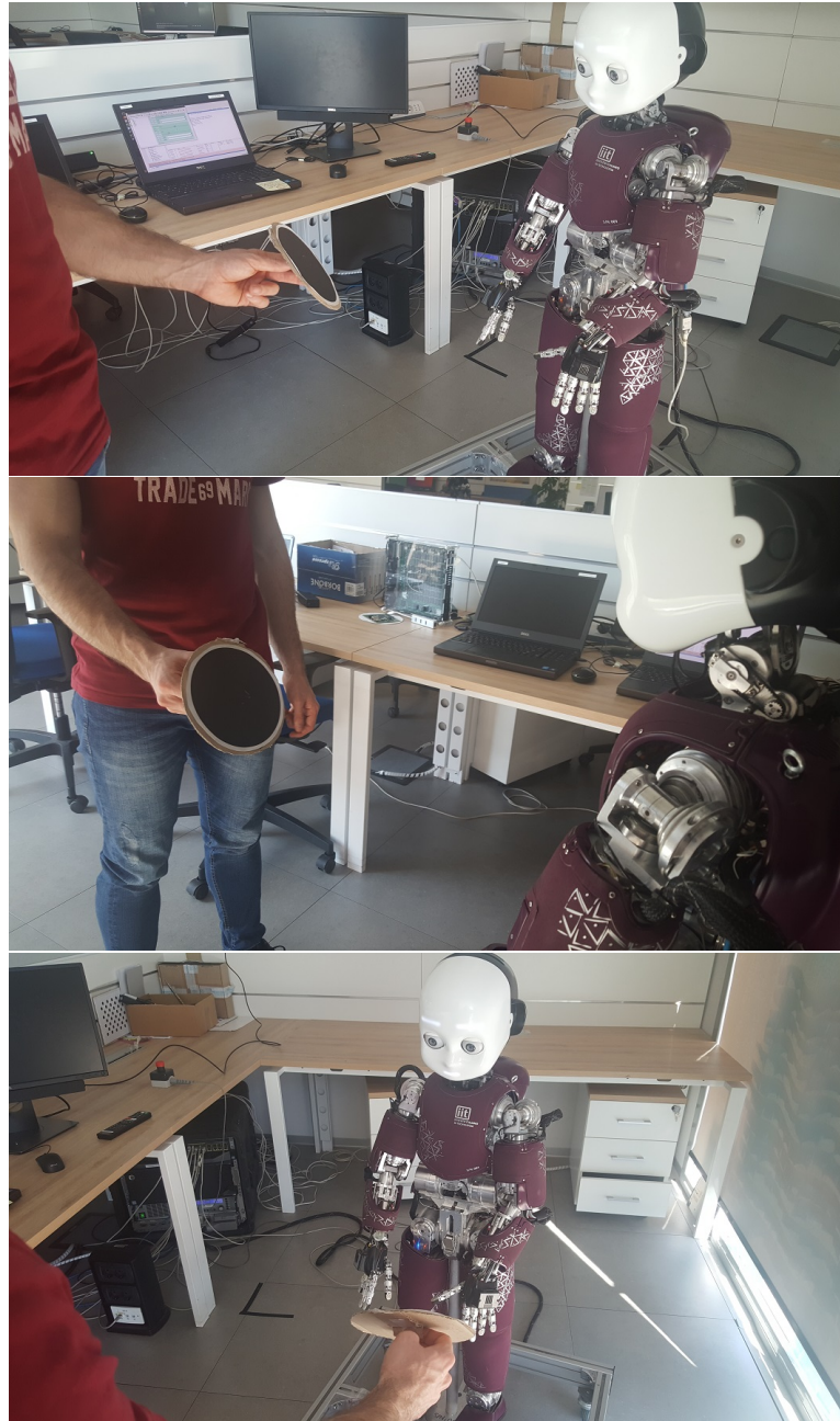
Figure 2.2: The task considered in this work is a kind of handover task, where the person in front of iCub is handing an object to the robot, but can also retract the hand. This can be useful in future work to plan different behaviors for the robot.
