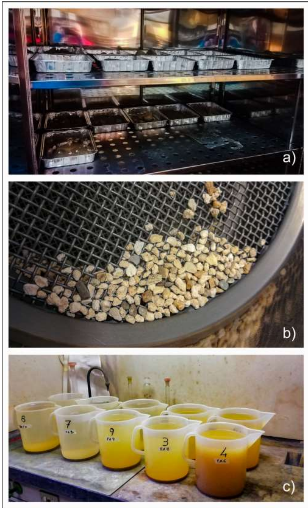
Figure 29 - Various steps of grain size determination procedure are shown. a) The samples are oven-dried. b) Subsequently sieved using different mesh sizes. c) Preparation of the fine fraction for the sedigraph (All pictures by me, except for the last one by Mr. Demergasso).
