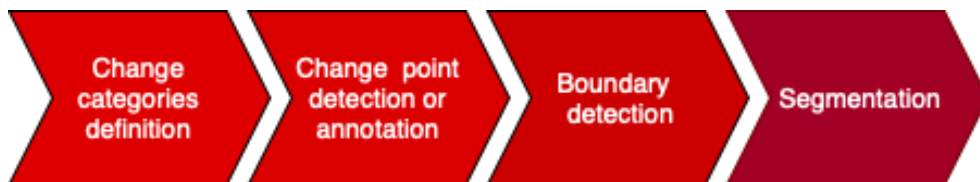
Figure 7: Workflow to achieve segmentation through our technique. Features from each change category are extracted either automatically or manually. After, boundaries are detected through CPD algorithms or via manual annotation. Boundaries are then combined and segmentation is performed when boundaries from different change categories align.
