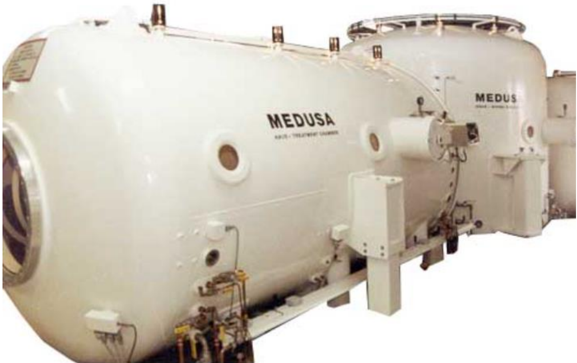
Figure 3-6. Medusa simulator for saturation diving training.
