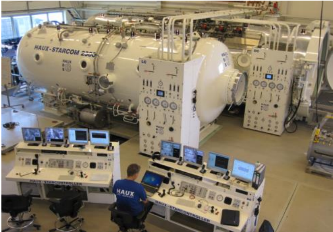
Figure 3-5. HAUX simulator for saturation diving training.
