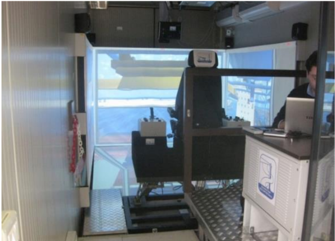
Figure 3-8 Port crane operator workstation mock-up on motion platform
