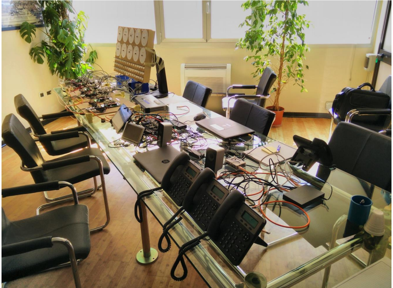
Figure 8-8. Testing control panel, atmospheric monitoring measurement equipment and communication system
