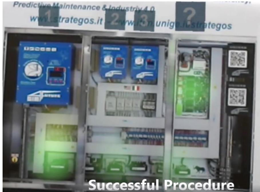
Figure 3-16 Capture from Microsoft HoloLens: launch sequence (numbers) is overlapped with the control panel mock up
