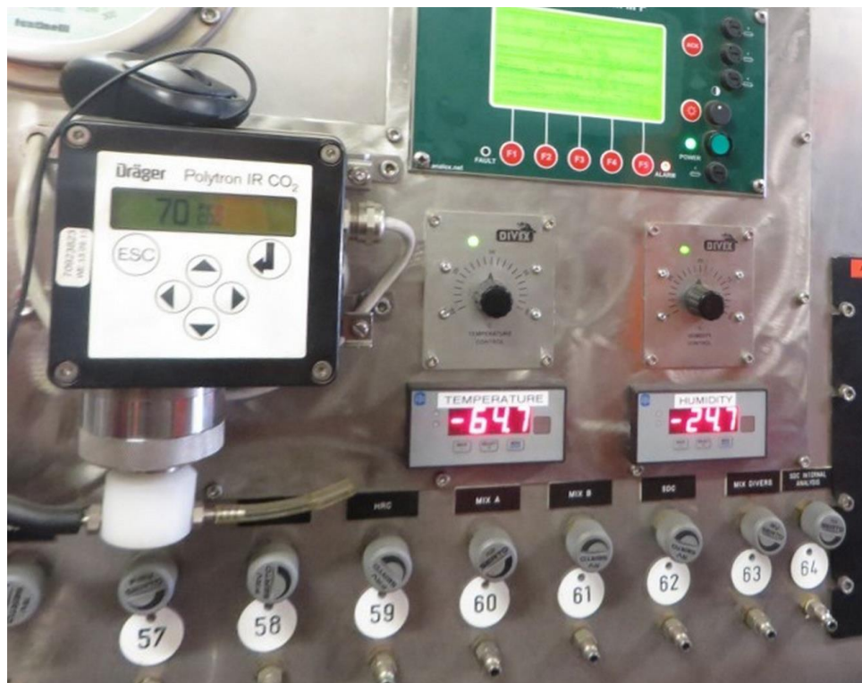
Figure 2-8. Polytron Dräger CO2 Analyser and connectors to the chambers.
