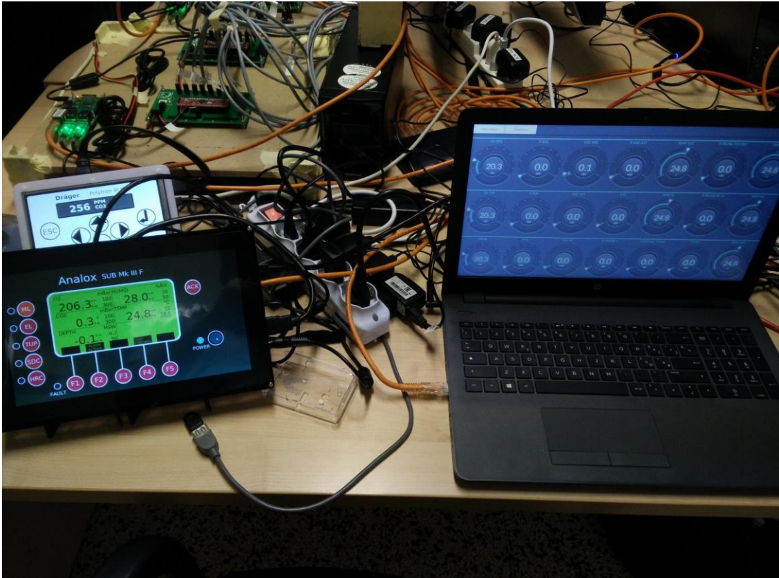
Figure 7-9. First integration test combining prototypes of 3 atmospheric monitoring systems and analysers and mock-up of valves and pressure gauges
