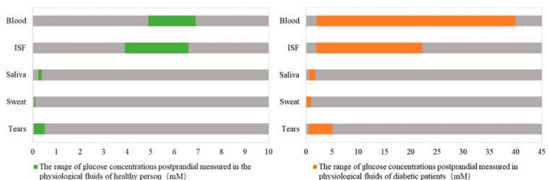
Figure 1.13 Contrast of glucose concentrations in different physiological fluids between healthy and diabetic people 108 .
