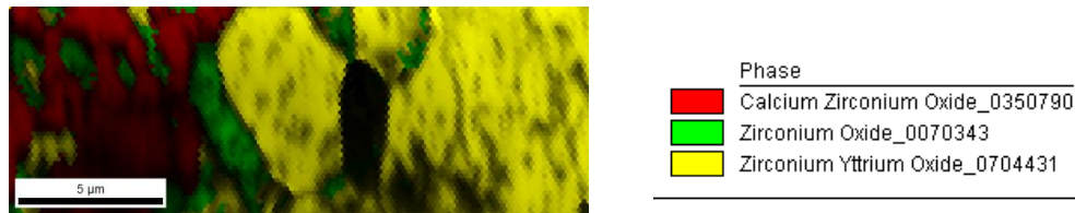
Figure 20 - Example of phase map obtained with monoclinic phase exposed for 1000h at 1200°C
