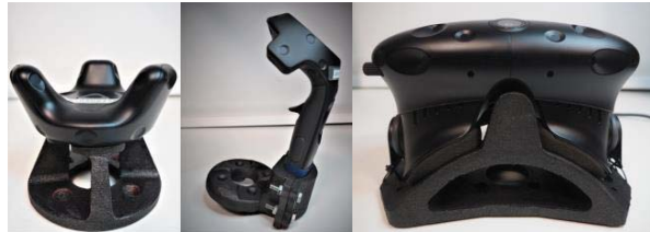
Figure 4.4 Vive tracking devices with their 3D printed mounts for flange ISO9409-1-A63. From left: tracker, Controller, and HMD.
