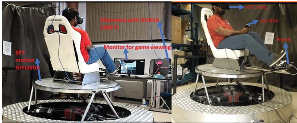
Figure 3.1 SP7 flight simulator set up with the user on the platform.
