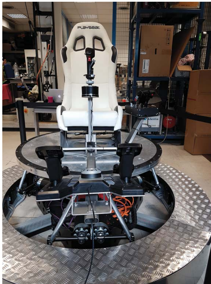
Figure 2.8 SP7 motion simulator with flight simulator gears.
