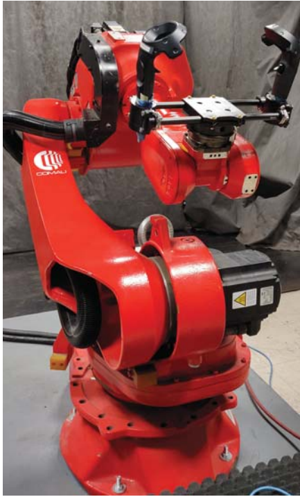
Figure 4.3 Ground truth system: Comau NS16 1.65 foundry hand robot with the mount for controller dynamic analysis attached to the end-effector
