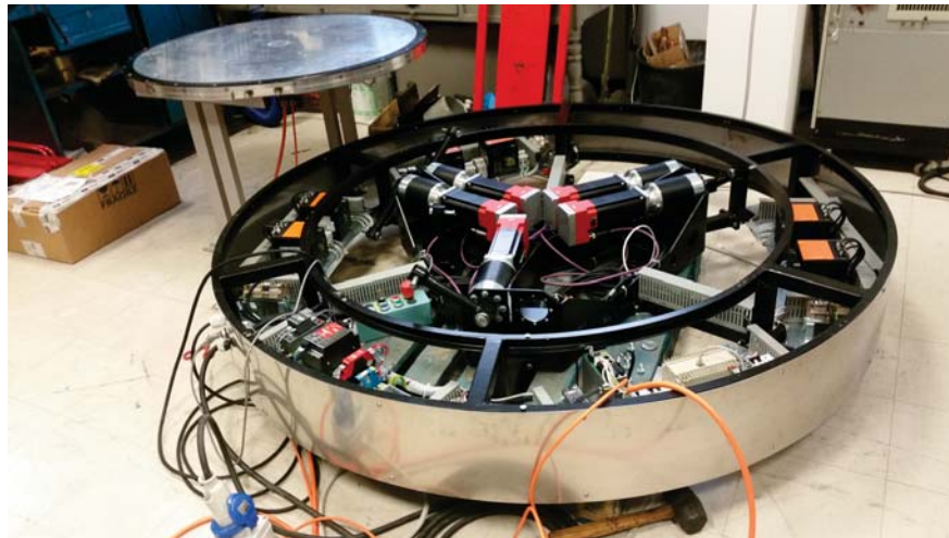
Figure 2.12 Disassembled SP7 platform with the actuators and controllers in view.
