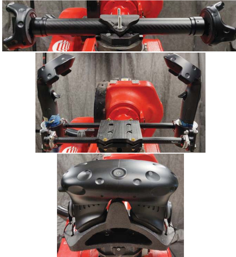
Figure 4.5 Metrology bar, with devices on both ends and its C16 tool mount. Top: A 350 mm long carbon fiber tube, with VLTS's tracker on both ends. Middle: An assembly of two carbon fiber rods and rack, with VLTS's controller on both ends. Bottom: HMD mounted on the end-effector of C16.
