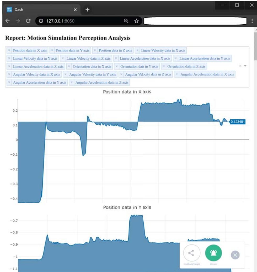
Figure 5.3 Real-time post-processing of tracker data using Python-Dash
