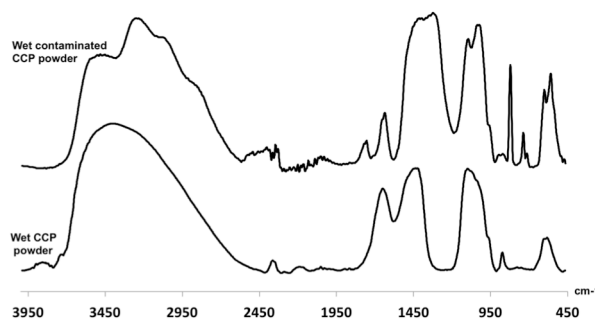
Figure 5. FTIR PAS of wet poor and wet contaminated CCP.
