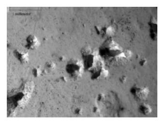
Fig. 1. Light microscopy of HAp ceramic surface
