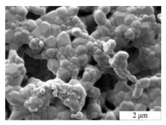
Fig. 2. Scanning electronmicroscopy of HAp ceramic
