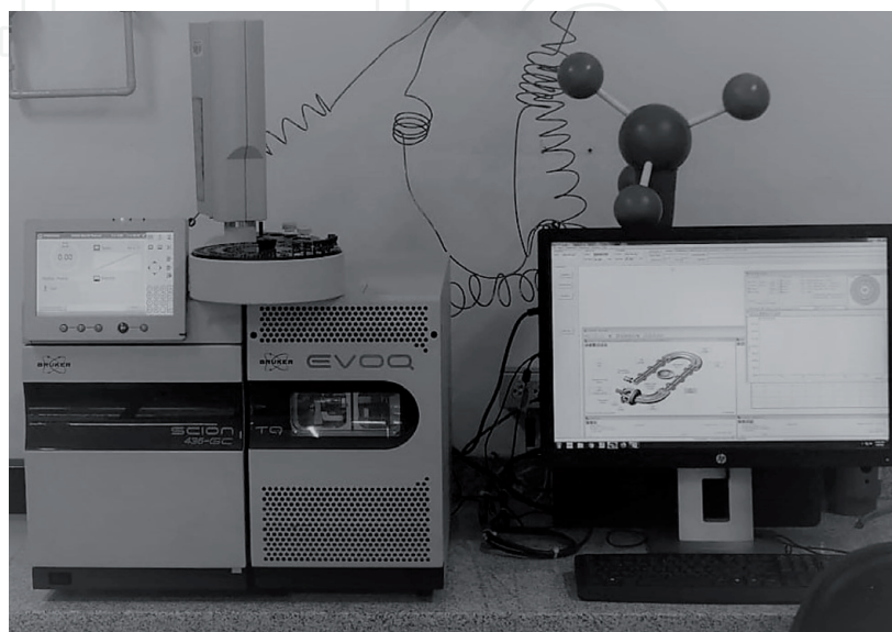
Figure 4. Gas chromatography equipment coupled to mass spectrometer. Life Sciences Laboratory, Salesian Polytechnic University.
