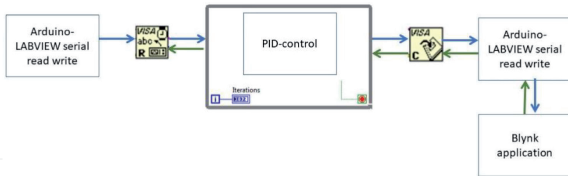
Figure 3. General visualization block for software dataflow in remote monitoring.
