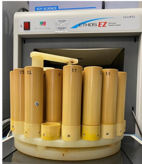
Figure 2: Picture of the Milestone Ethos microwave digestion system used in the study
