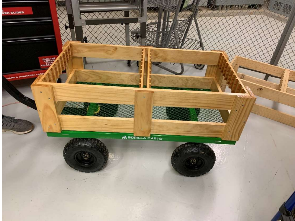
Figure 14: Completed Final Prototype w/ Side Supports
