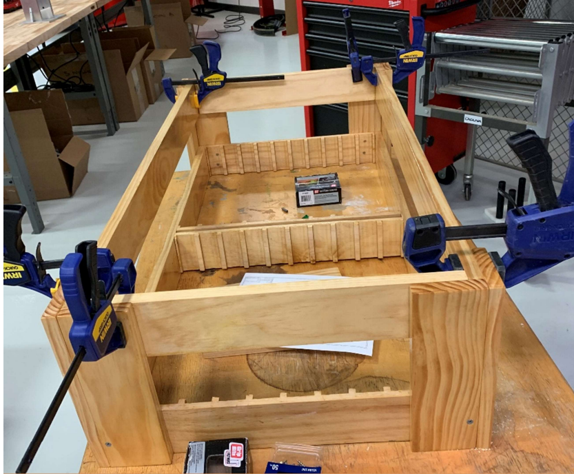
Figure 13: Clamped “Bottom” of Wagon Frame
