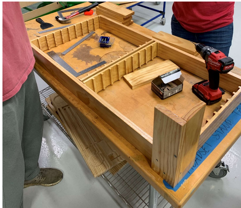
Figure 17: First corner support assembly
