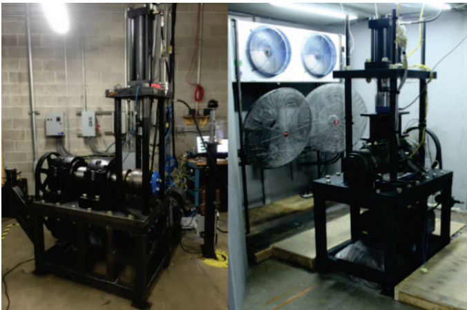
Figure 3. Single bearing test rig (left) and four-bearing test rig (right).
