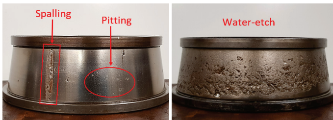
Figure 2. Examples of localized defects (left) and distributed defect (right).
