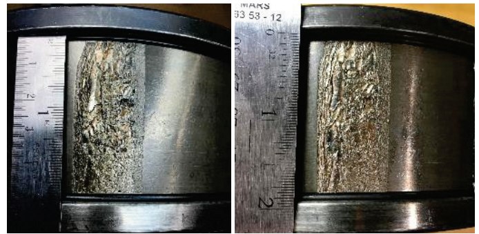
Figure 12. Initial cup spall (left) and final cup spall (right) for Experiment 202. [ruler in inches]
