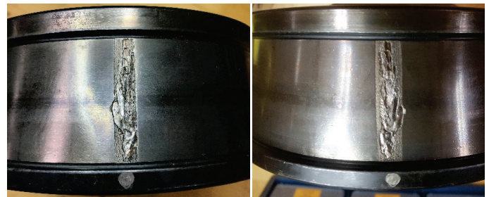
Figure 10. Initial cone raceway spall (left) and final cone spall (right) for bearing B2 in Experiment 209.
