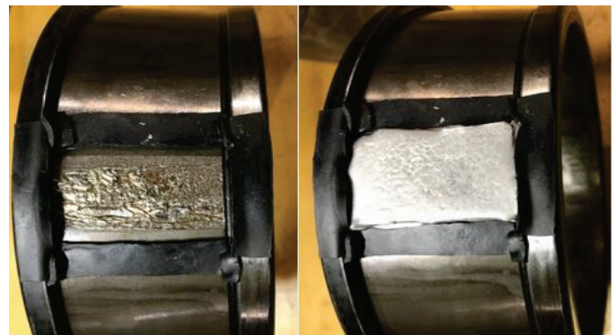
Figure 8. Casting procedure using bismuth and sealant tape
