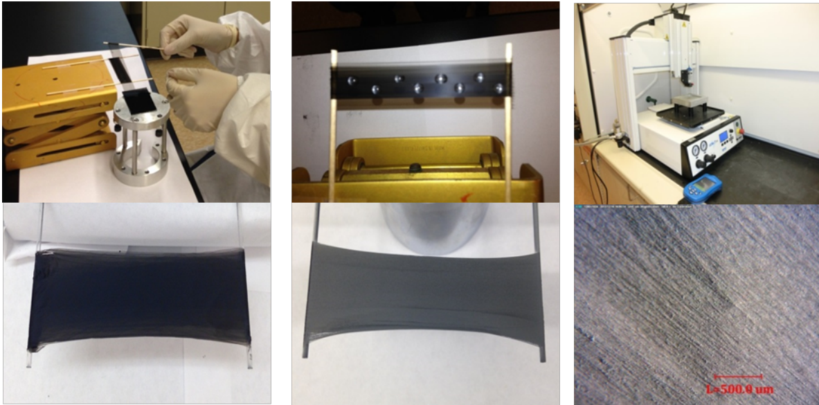
Figure 6. Preparation of MWCNT sheets, and coating with NGG using robot EFD-325TT equipped with a Paasche VL-SET airbrush system.
