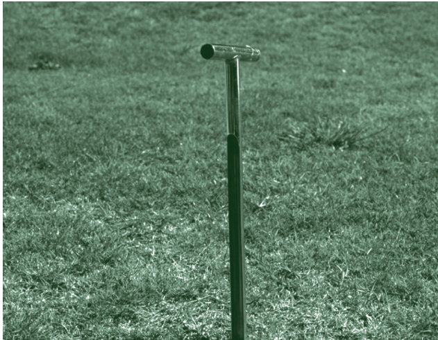
Figure 4. A "T" type soil sampling probe is the best tool for collecting nematode samples.
