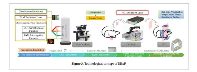
for both all-optical detection photoacoustic interrogation and optical coherence tomography (OCT) at 780 and 1310 nm with wide bandwidth, narrow linewidth, and stable phase.
