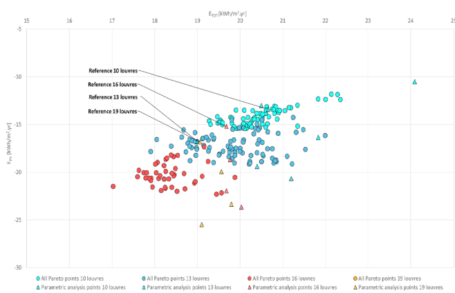
Fig. 7. Visualization of the Pareto points from the optimization study with regard to energy use and PV conversion.
