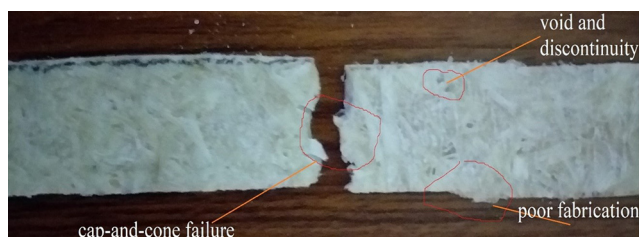
Fig. 5. Failure type for tensile specimen.
