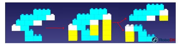
Figure 3.12: Another example from Sugimote et al.'s thesis recreated in RoboDK, this example combines both support blocks and sub-figures to build a difficult shape
