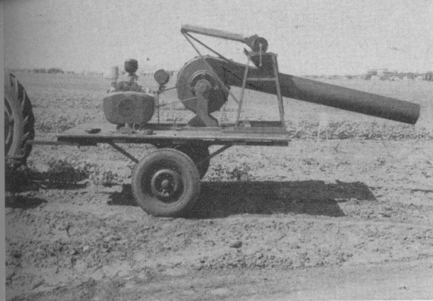
Figure 6. A machine that was made to inflict hail-like injuries by blasting plants with cracked ice (left). An example of heavy damage caused by the hail machine in June at Lubbock (right).
