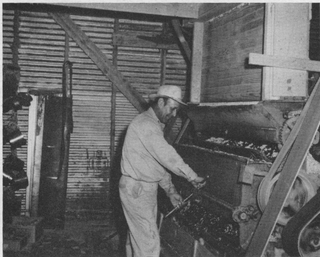
Figure 5. Cotton planting seed coming through a delinting stand. Courtesy of Northern Star Seed Company, O'Brien, Texas.
