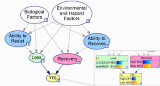
FIG 1. Proposed BN template for analysing cumulative effects for a given metric of interest, Y(t), showing the factors as nodes, and dependencies as arrows. Shown in the inset are the outputs of the BN, represented as beliefs for the loss, recovery and Y(t) nodes (e.g. the probability of 0 to 25 units of loss occurring is 53%).
