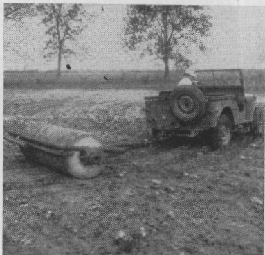
Fig. 8. The military jeep pulling a solid concrete roller weighing approximately 6,000 pounds over fairly firm soil. The drawbar pull was 750 pounds. On soft freshly disked land the pull will be much more.
