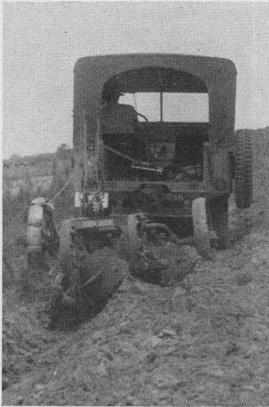
Fig. 6. The Universal jeep hitched to a plow equipped with two 14-inch general purpose plow bottoms. The drawbar pull was 1400 pounds which was an overload for the jeep.
