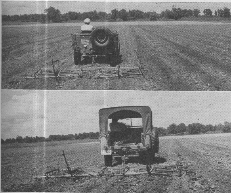
Fig. 5. The military (top) and Universal (bottom) jeeps pulling a two-section spike tooth harrow.
