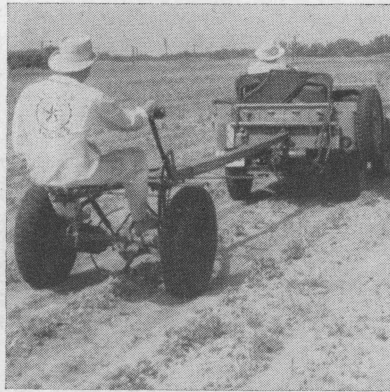
Fig. 10. The Universal jeep pulling a single-row cotton chopper. It could easily pull a four-row chopper.
