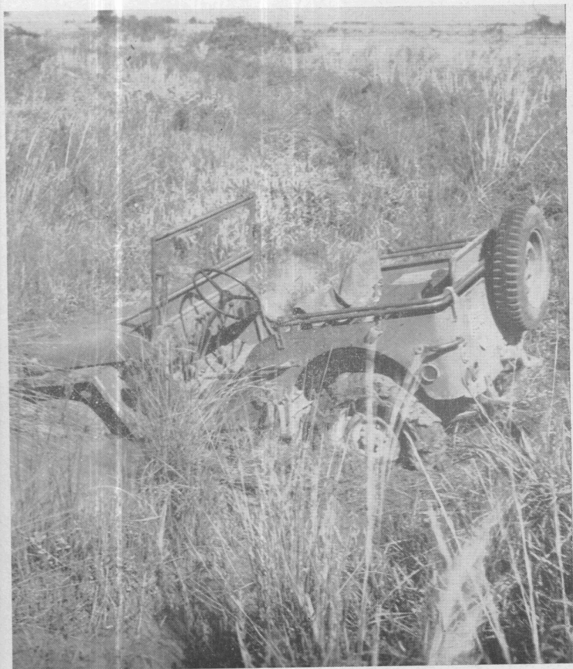
Fig. 22. The jeep cannot go everywhere. An attempt was made to cross a drainage ditch on a rice farm. The soft mud in the ditch was too deep and the jeep sank to where the tops of the front wheels were almost covered.
