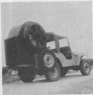
Fig. 16. The Universal jeep used as a truck to haul a large fan weighing about 725 pounds.
