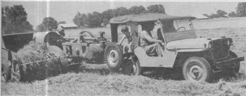
Fig. 11. The Universal jeep pulling a small pick-up hay baler. A total of 100 bales of hay were baled in one hour.
