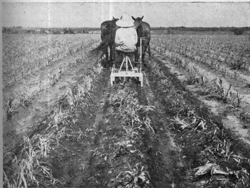
Figure 10. Garlic digger in operation. This digger had a U-shaped blade that cut the roots and loosened the soil around the bulbs so they could be lifted. The leaves and bulbs lost some moisture and became partially cured when left in dry soil for a few days, following the use of the digger.
