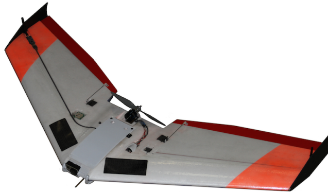
Figure 2.3. The ARSENL ZephyrII fixed-wing UAV. Source: [8].
