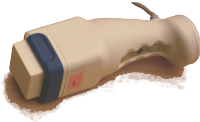
Figure 2.12: Illustration of a CZT-based hand-held gamma camera (Knoll et al., 2015; Roth et al., 2020). The left end of the device is a parallel-hole collimator with a front area of approximately 4 \times 4 \text{ cm}^2 .
