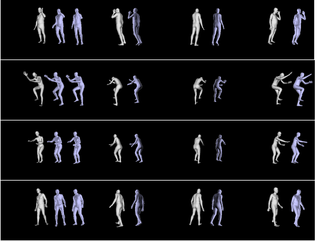
Figure 2.4: The figure shows results on synthetic data. Each row corresponds to one person with some unknown shape and pose. For each row the left hand image in each column is the input image for frame one to four. The middle image in column one is the result from SMPLify using only the input image from frame one. The right hand image in each column is the result of our method using all four input frames.
