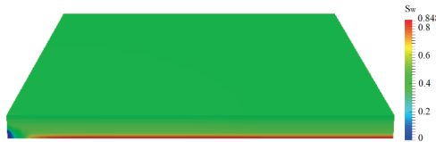
Figure 4.13 The distribution of water saturation for the reservoir with a residual water saturation of 0.55 (gradually increase from approximately 0.46 to 0.85 from the top layer to bottom layer result from the flowing downward of flowable water dominated by gravity)
