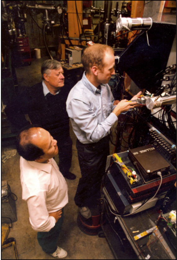
Charles Barnes and research fellow T. R. Wang look on as research fellow Stephen Kellogg inserts a fusion cell array into the neutron detector, in their attempt to replicate the Pons-Fleischmann cold fusion experiment. Caltech Archives
