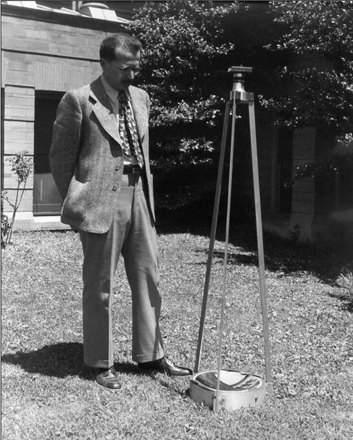
Jesse Greenstein stands beside the wide-angle camera he designed with fellow Yerkes astronomer Louis G. Henyey in the late 1940s. A spherical concave mirror with 12-inch aperture is surmounted by three struts supporting a multi-component lens. The camera covered a field angle of 140^\circ with critical definition and produced photographs similar to naked-eye observations. Today's "all-sky" cameras are largely the progeny of the Greenstein-Henyey device.*
