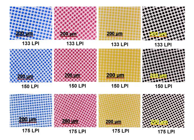
Fig. 3: Dot structure for CMYK at varying plate resolutions
