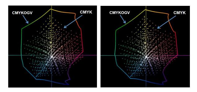
Fig. 7: Gamut Comparison between CMYK and CMYKOGV with 728 patches (left) and 2016 patches (right)
