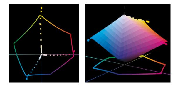
Fig. 5: 2D Plot (I) and 3D Plot (r) of Optimization Run (CMYK) Vs. CRPC 6 GRACoL 2013 Profile
