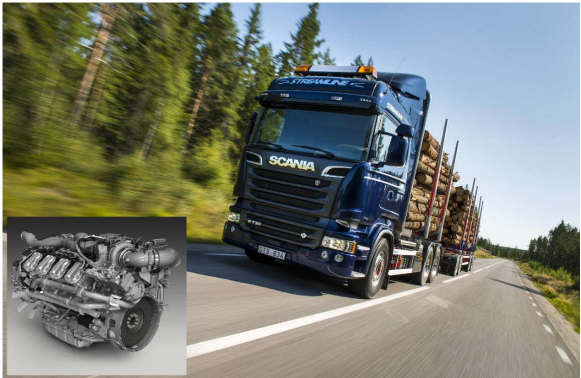
Figure 5.6: Scania R-730 with 16-litre V8 520/580 horsepower Euro 6 engine, fitted for timber (Scania, 2013)
