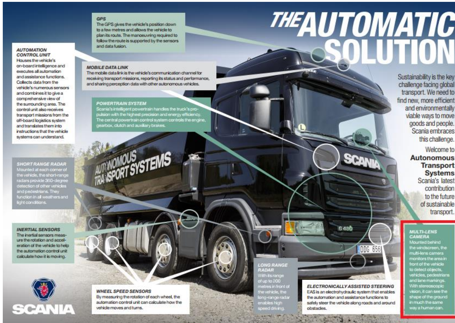
Figure 5.11: Multi-lens camera system featured in next-generation Scania HGVs
