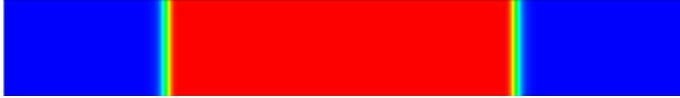
Figure 7- Flat interface simulation to test thermodynamic consistency (Colour illustrates density).
