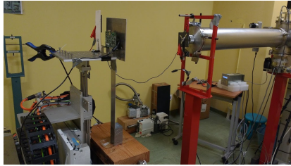
Figure 1.5: Experimental setup using proton and neutron irradiation test.
