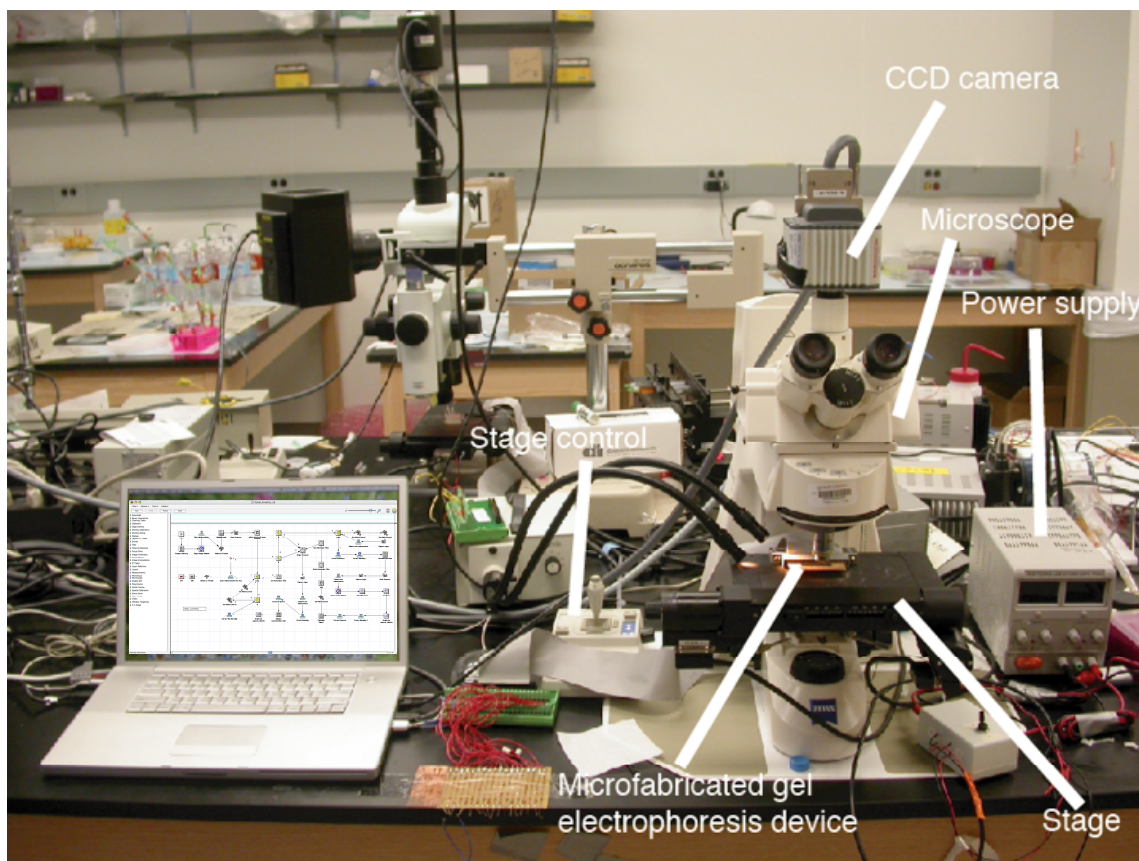
Figure 13. Experimental set-up showing the optical microscope with the attached CCD camera and stage control interfaced to the computer. Automations developed in-house using the Openlab software (Improvision Inc.) control the image capture and analysis in real time.
