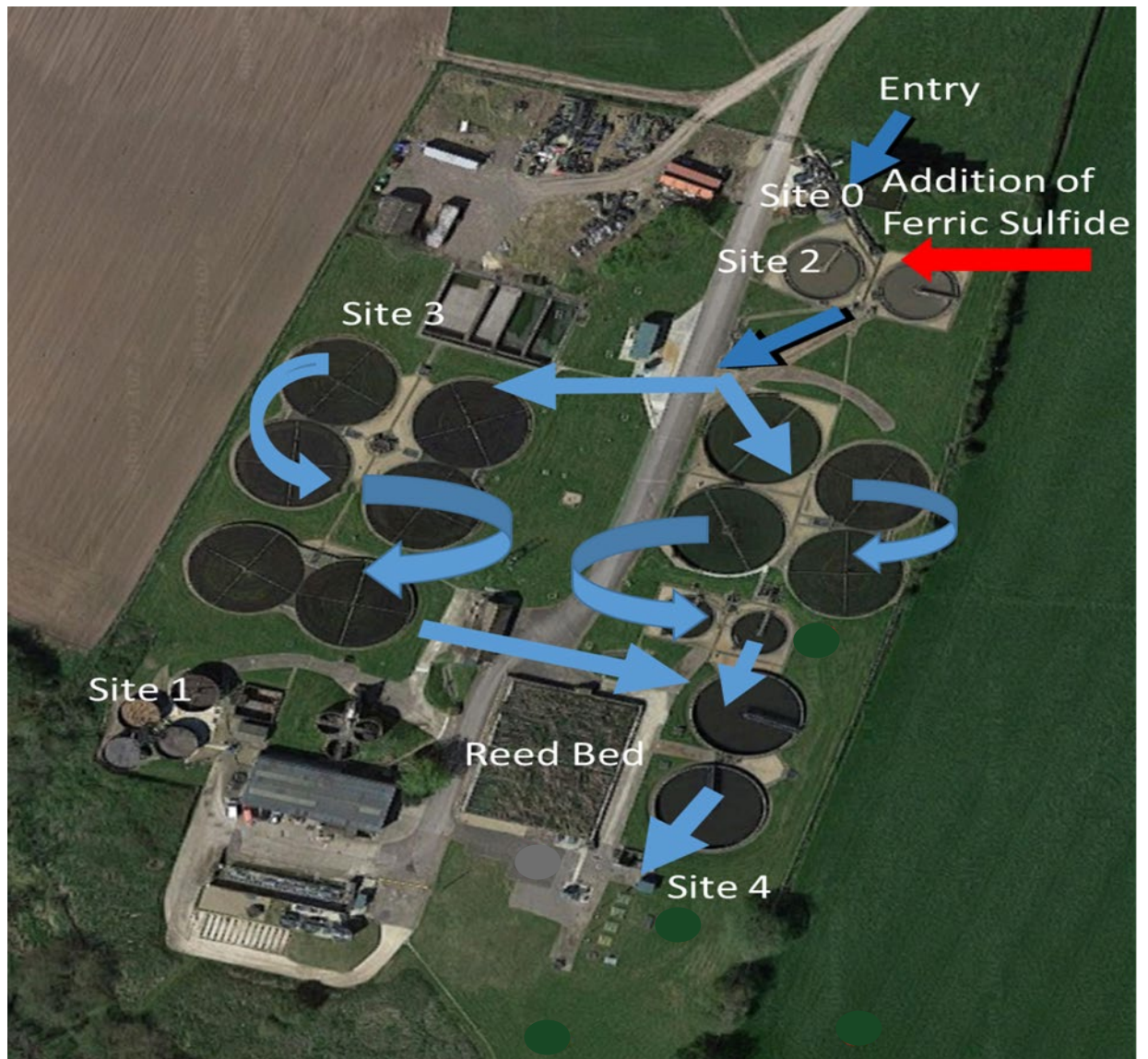
Figure 9. Schematic view of Petersfield Water Treatment plant. Untreated Effluent enters at Site 0 and is screened. Water containing more dense particles removed and taken underground to Site 1 for sludge processing independent from the rest of the plant. The remaining water moves through a pipe where ferric sulphide is added. The large volume of water is split in half into site 2 and site 3, for ease of processing before it is moved to the start of a series of trickling filters. The contaminated water is spread, via mechanical rotating arms, over basins containing large stones. Aeration of the water favours the breakdown of organic materials as it is passed over biofilms present on the gravel. Water is then passed through a holding tank (Site 4) before ejection into the surrounding environment. The reed beds are used to handle overflow, resulting when the rainfall is heavy. This provides some treatment before the water is released.
