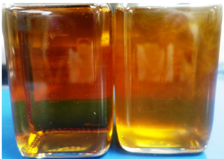
Fig. 9. Freshly prepared Brij® C10-based PD working solution showing a clear appearance (left) and Tween® 20-based PD working solution showing slight cloudiness (right).
