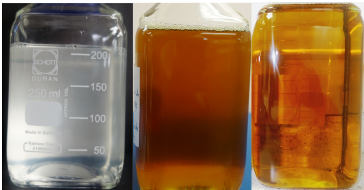
Fig. 4. Photographs of cloudy solutions; Tween® 20 stock detergent (left) and Tween® 20-based PD working solution (middle), and a clear PD working solution using Synperonic® N (right).
