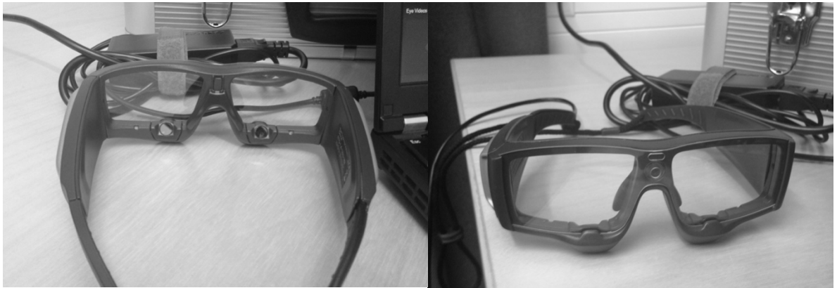
Figure 2.6: Example of a head mounted eye tracker: The SMI 2.0 Glasses (Discombe & Cotterill, 2015).
