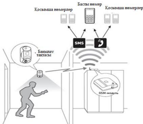
Figure 1 – Principle of operation of the GSM alarm system
