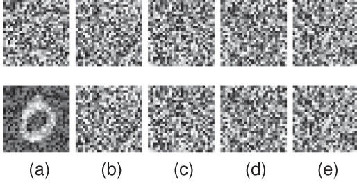
Fig. 5. An example of splitting an image in the MNIST dataset into two shares with regard to different choices of n . One share is in the top row and the other is in the bottom row. (a) n = 8 ; (b) n = 16 ; (c) n = 24 ; (d) n = 32 ; (e) n = 40 .
