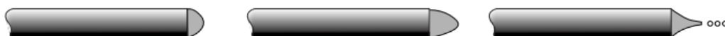
Figure 1.2 The formation of electrospray. Left: at a low voltage, the drop is almost spherical. Centre: with a higher voltage, but below the onset potential (1-2 kV), the drop elongates under the pressure of the charges accumulating at the tip. Right: at onset voltage, the pressure is higher than the surface tension, drop shape changes to a Taylor cone and small droplets highly charged are released. (Adapted from Dass 2007).
