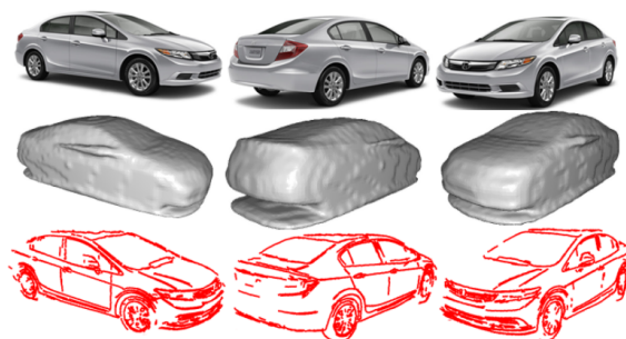
Figure 3.12: Stages for the development of a vehicle's 3D model used by Ramnath et al. (2014). Top: three of the images used to generate the hull; centre: visual hull; bottom: 3D space curves projected into the visual hull. (Retrieved from [152].)
